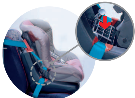
The belt is tensioned automatically.
